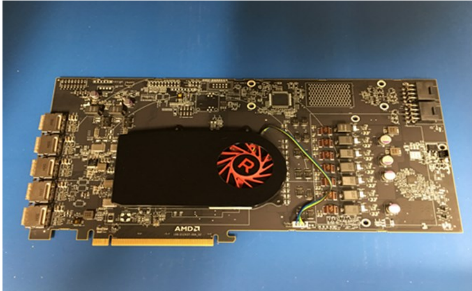
Figure 3: PCIe Development Board
