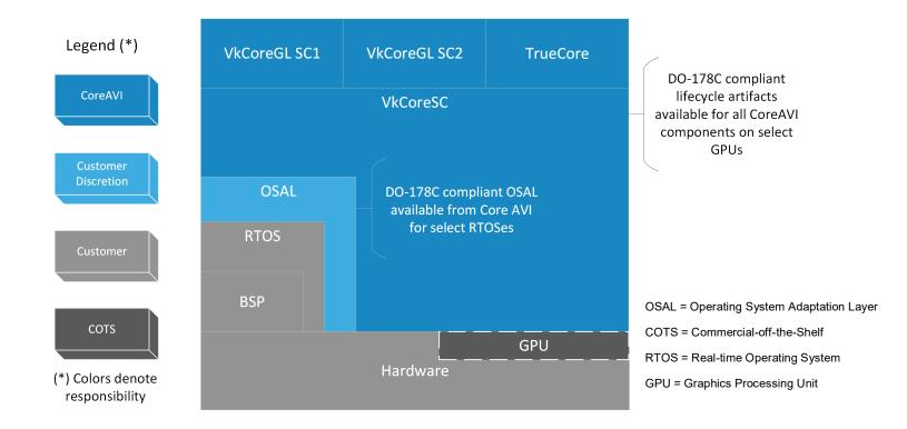
CoreAVI uses an Operating System Adaptation Layer (OSAL) architectural approach to isolate OS-specific function calls into a single layer and simplify porting between operating systems.
