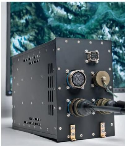
This solution enables system integrators and end-users to leverage the high-resolution imagery provided by aircraft-installed sensors and available databases as well as large area displays to be installed in future aviation cockpits. Thus, the HENSOLDT Mission Computer with CoreAVI graphics drivers is already supporting the requirements of tomorrow's avionic architectures.
