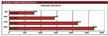
Note 1. e/m indicates the 3D engine (e) and memory (m) clock speed in MHz
