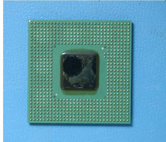
Figure 3 External bottom view of subject device after 8 hour steam age
