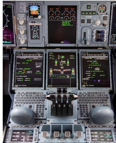
The Airbus A380 cockpit display system employs AMD ATI Radeon GPUs, EASA ED-12B safety certified OpenGL and several COTS safety critical operating systems.
