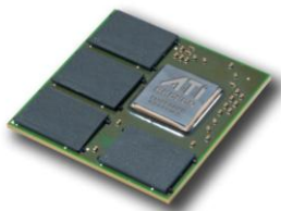
Temperature-screened versions of AMD's ATI Radeon E4690 are available with 20-year supply programs from Core Avionics & Industrial (a Channel One Company).
